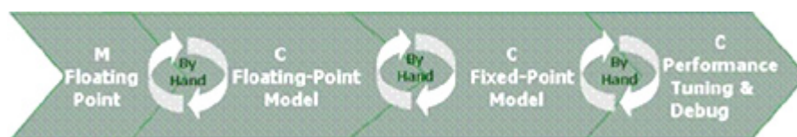
Figure 4 — DSP application development flow
